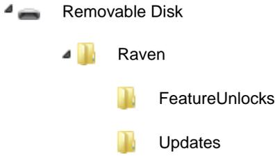
A “Raven” folder must be created on the root directory of the flash drive. Inside the Raven folder, create an “Updates” folder for Software Updates and a “FeatureUnlocks” folder for software feature unlocks as shown in the figure above.
