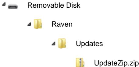
Once the flash drive is inserted into the Viper 4, the .zip file containing the software update will be copied into internal memory and extracted automatically. Once this process is complete, the software update will be available via the System Manager utility within the Software Update tab.
