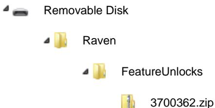
5. To apply the software unlock, insert the flash drive into the Viper 4. After a short time, a message will be displayed prompting the operator to restart the field computer. Remove the USB flash drive before restarting the Viper 4.
